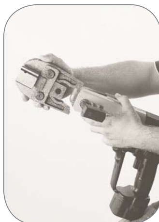
Place the jaws in the housing
